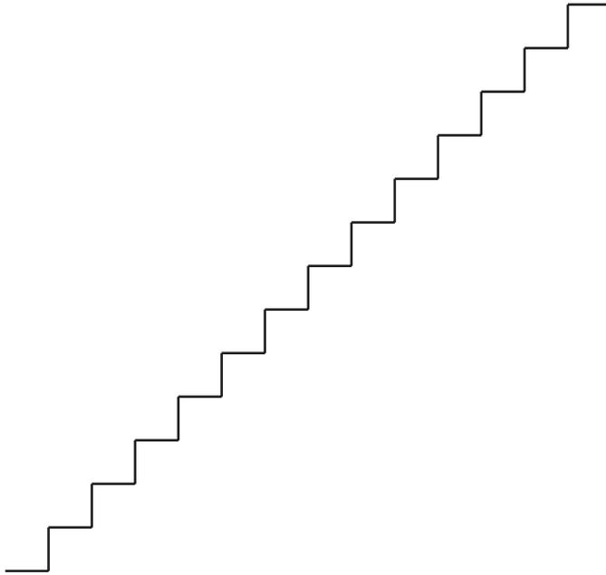
**Figure Z.3** An analog signal is smooth and continuous. A digital signal is stepped as the value changes. Zipper noise results when a digital control signal lacks resolution to smoothly change a parameter.
