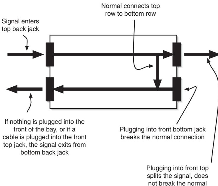
**Figure N.4** Plugging a jack into the top front jack on a half-normalled patch bay will result in a signal split. Plugging into the lower front jack interrupts the signal.
