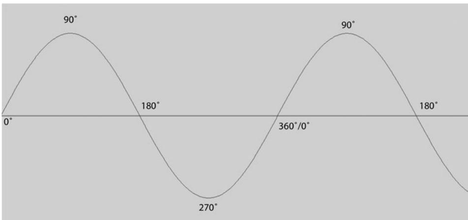
**Figure P.7** A wave’s phase is a point in its cycle in relation to time.
