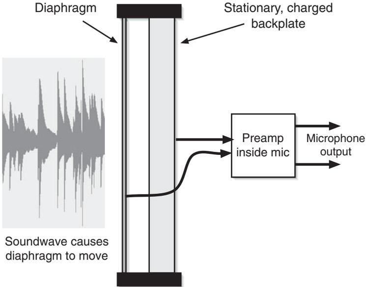
**Figure B.1** The output signal in a condenser microphone results from the motion of the diaphragm in relation to the backplate.
