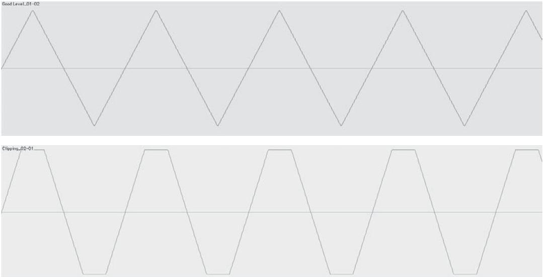
**Figure C.4** Clipping occurs when a signal exceeds the maximum level that a circuit can pass without overloading. Higher levels will result in the top of the waveform being squared off and distorted (bottom).
