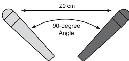
**Figure D.7** With the DIN stereo mic technique, two cardioid microphones are positioned 20 cm apart, at a 90-degree angle.
