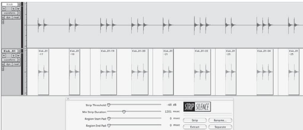
**Figure 5.20** When a strip silence-type function is used, audio below a threshold level is removed, and the remaining audio is broken up into separate regions.
