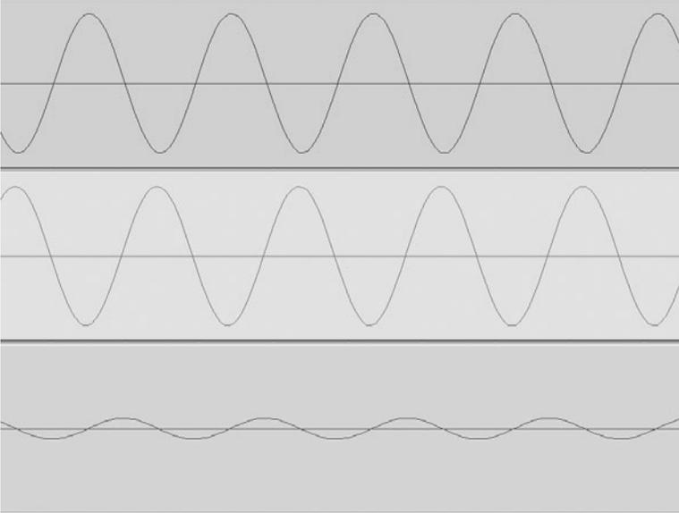
**Figure P.8** Two waves that are out of phase will cancel each other to some degree. If they're 180 degrees out of phase, they will cancel completely.
