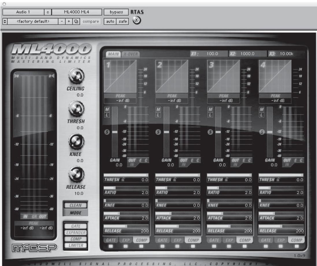
**Figure D.11** A multiband compressor is a type of dynamic equalizer that can dynamically change the levels of different frequency bands in response to input levels.
