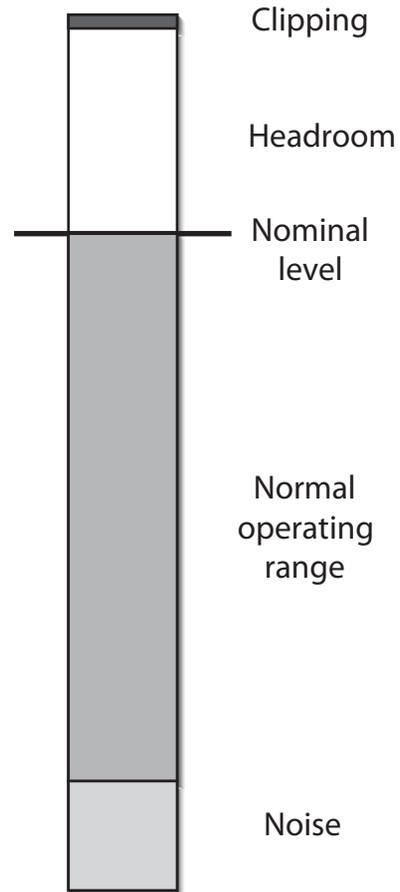
**Figure H.2** Headroom is the dynamic range above a device's nominal level and below clipping.
