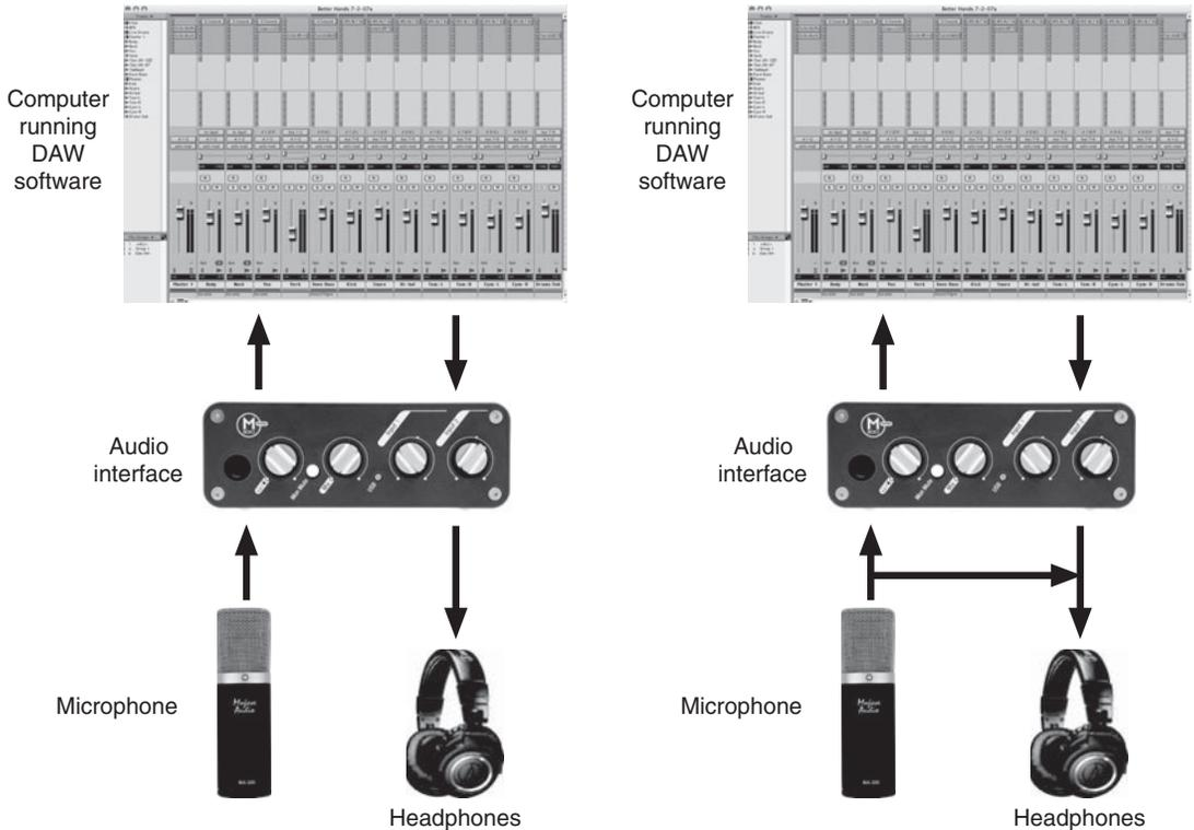
**Figure Z.2** When recording with computer-based systems, the signal must enter the audio interface, pass through the computer/software, and come back out through the audio interface—all of which takes a certain amount of time (left). Some audio interfaces, however, have a feature that allows signal from the input to be fed straight to the output, eliminating the delay (right).
