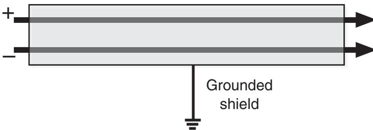
**Figure B.2** A balanced audio signal has positive and negative signals that are added together, canceling any noise picked up by the cable. A grounded shield surrounding the two conductors also helps to protect against noise and interference.
