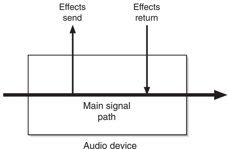
**Figure E.2** An effects loop provides a way to insert an effects device or processor into a piece of gear's signal path.
