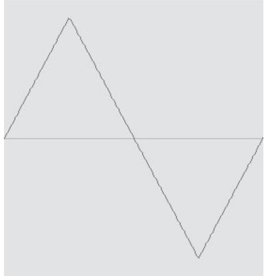
**Figure C.13** A cycle is one complete positive/negative repetition of a waveform.
