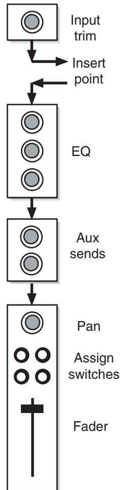
**Figure I.2** An insert point can be used to interrupt a mixer channel’s signal path so that an external processor can be applied to the signal.
