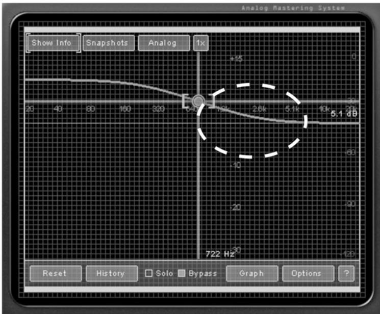
**Figure S.8** The skirt contains frequencies that extend beyond the bandwidth selected. In this case, the dashed circle shows the skirt that extends beyond the cutoff frequency of a low-shelf filter.
