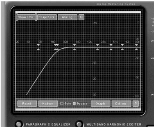
**Figure P.5** The range of frequencies in a signal not affected by a filter is called the passband.
