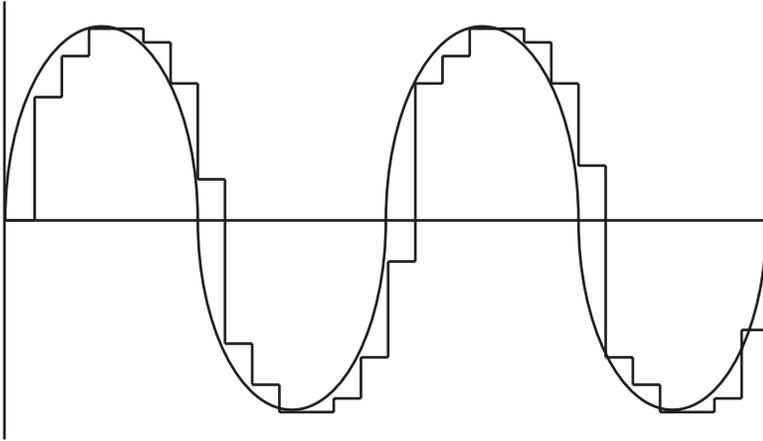
**Figure 5.17** The discrete values of a digital representation result in incremental stair-step changes rather than the smooth changes of analog.
