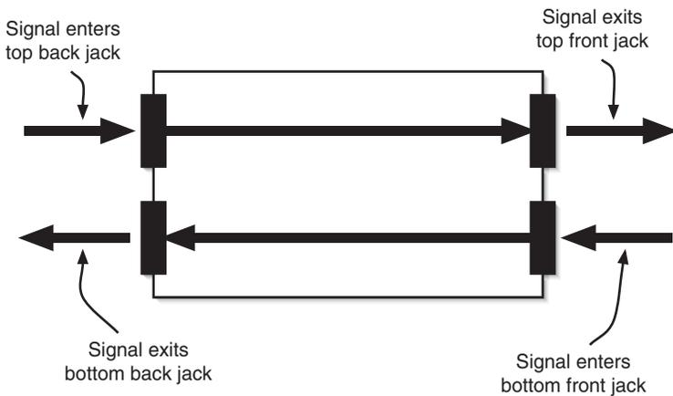
**Figure N.6** There is no connection between the top and bottom rows when a patch bay is open or non-normalled.
