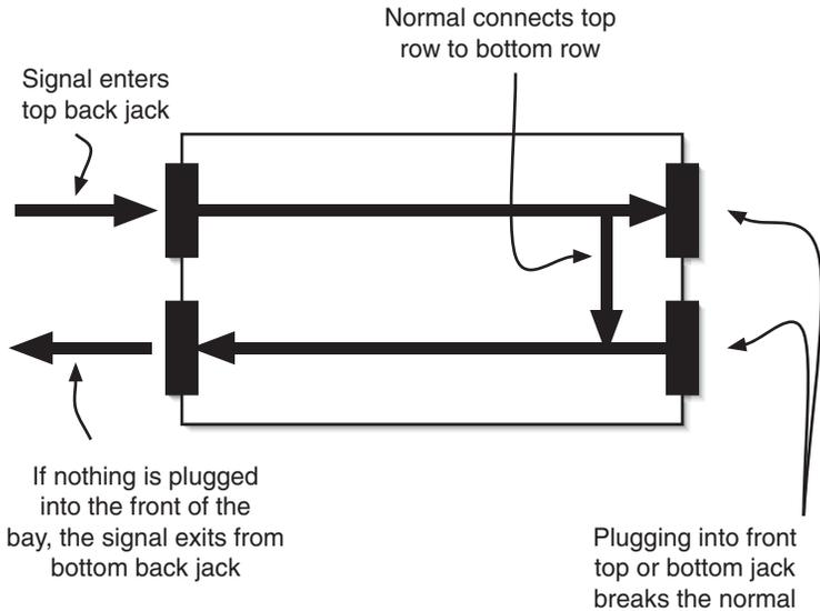
**Figure N.3** A full normal is interrupted if a cable is connected to the front top or bottom jacks.
