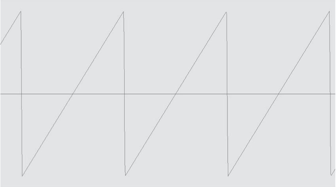
**Figure S.1** A sawtooth waveform contains a fundamental frequency plus all odd and even integer harmonics.
