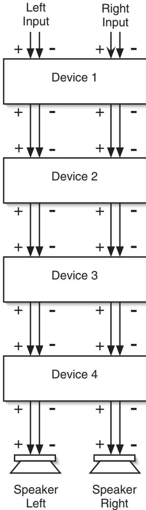
**Figure A.1** Positive and negative polarity are maintained throughout a system with absolute phase.
