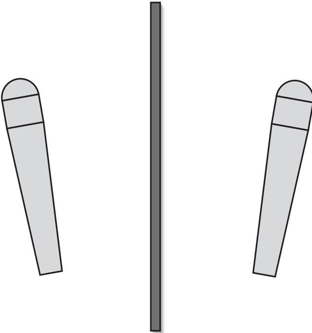
**Figure J.2** A Jecklin Disc is used to increase stereo separation when using two omnidirectional microphones. The microphones are placed 17 centimeters apart, angled out at 20 degrees, with the circular, absorptive disc centered between the mics.
