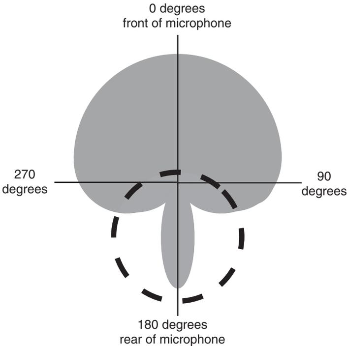
**Figure L.5** A section of a non-omnidirectional polar pattern bounded by a null is called a lobe. In this hypercardioid polar pattern, there is a lobe to the rear of the mic (circled in the figure).
