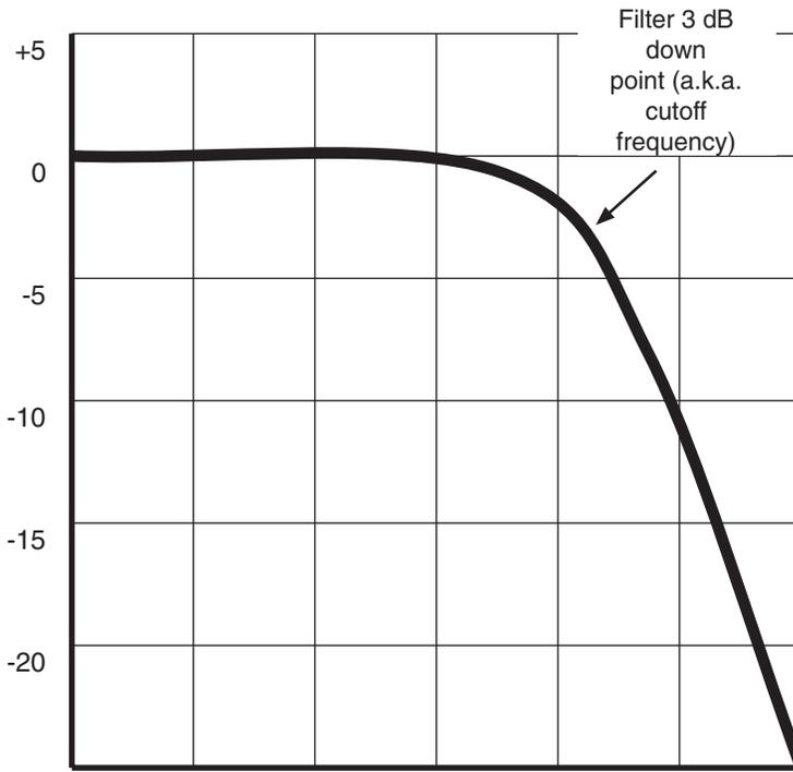
**Figure 1** A filter's (in this case, a low-pass filter)  $-3$  dB points are where the response of the filter is 3 dB below the passband.
