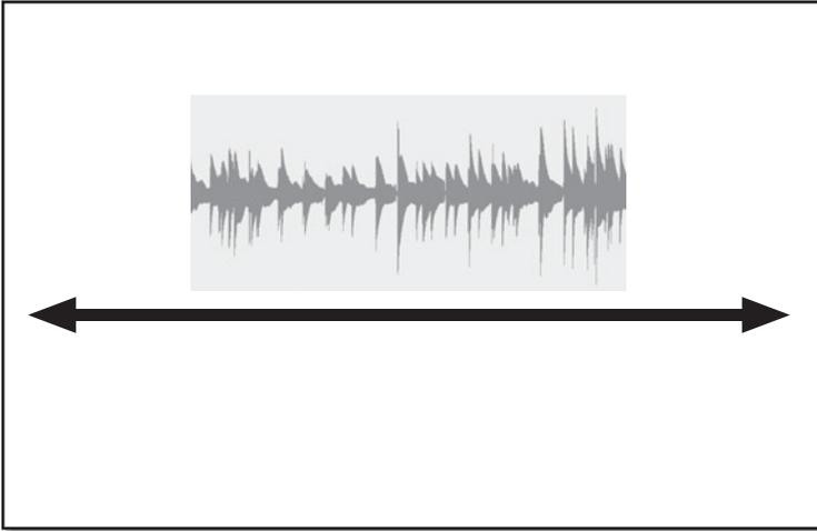
**Figure A.11** A sound reflecting between two parallel room surfaces creates an axial mode.
