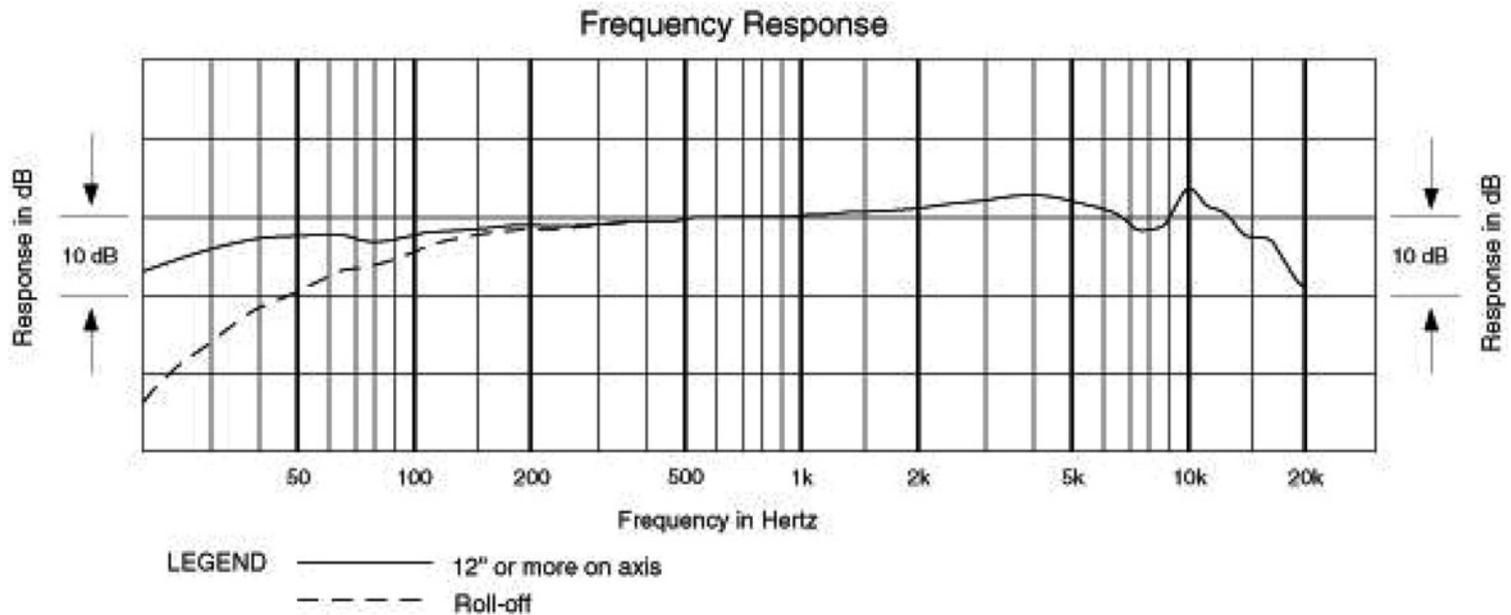
**Figure F.5** A frequency response curve is a graph of how well a device reproduces the frequency range. In this case, a microphone manufacturer has provided two curves, one (solid line) for the normal response, and the other (dotted line) for the microphone with low-frequency roll-off engaged.
