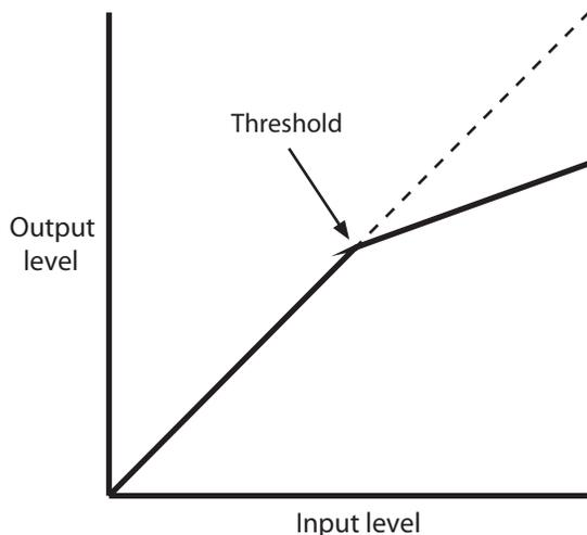
**Figure H.1** Most compressors use hard-knee operation, in which gain reduction is applied as soon as the signal crosses the threshold.
