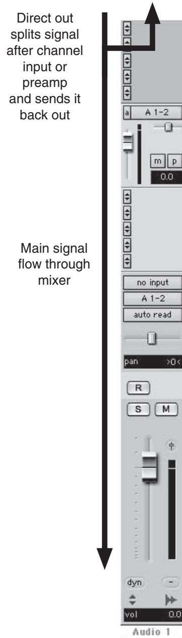
**Figure D.8** Direct outs on a mixer tap off the signal before it is bused and send it back out to another destination, such as a recorder or interface input.
