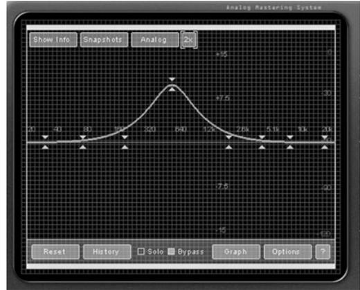
**Figure P.6** A peaking filter boosts a range of frequencies around a center frequency.
