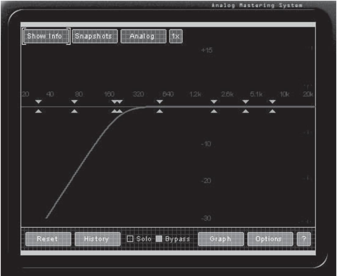
**Figure H.4** A high-pass filter allows frequencies over the cutoff frequency to pass unaffected, while reducing the level of frequencies below the cutoff frequency.
