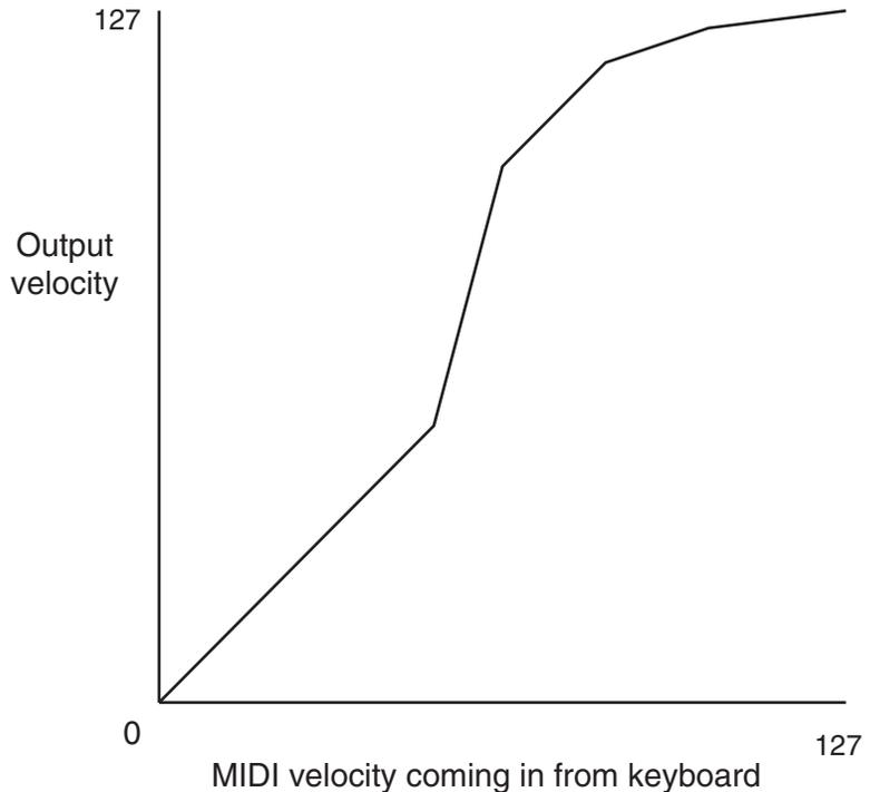
**Figure V.1** A velocity curve in a device can be used to customize the response or feel of the keyboard to match the player's touch.
