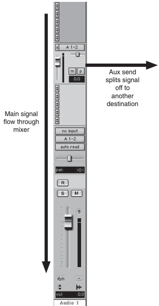
**Figure A.10** An aux send splits off signal from a mixer's main signal path and routes it to another destination, such as headphones or an effect processor.
