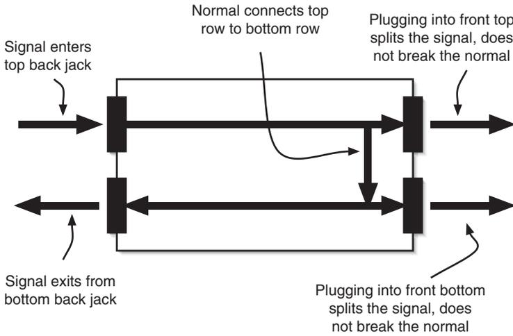
**Figure N.5** A mult works like a passive signal splitter.
