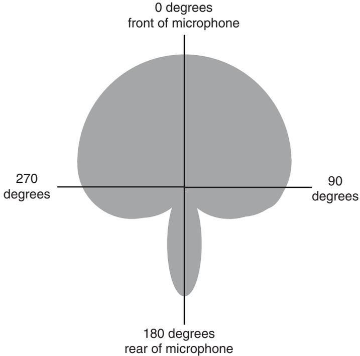
**Figure H.7** The hypercardioid microphone polar pattern is more directional than the cardioid pattern and has two nulls, creating a lobe to the rear of the microphone.
