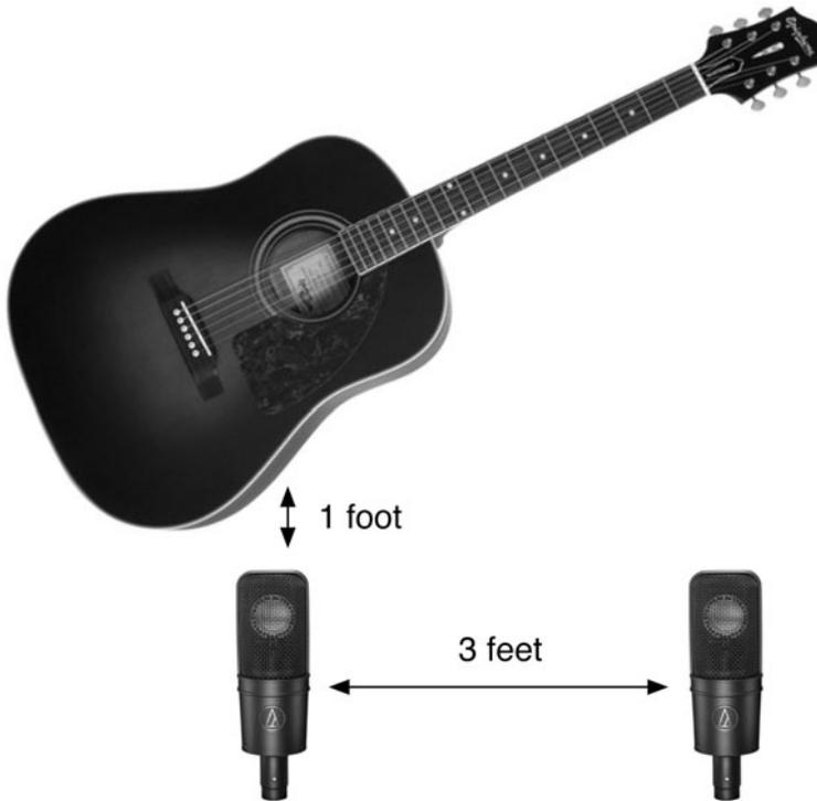
**Figure 2** The 3:1 rule for microphone placement says that when two mics are on a source, the second mic needs to be three times as far from the first mic as the first mic is from the source.
