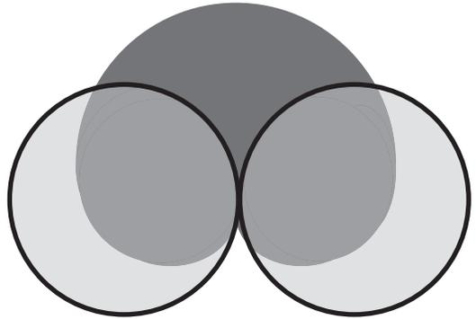
**Figure M.6** M-S stereo is a miking technique that uses coincident cardioid and figure-8 mics. It allows the engineer to adjust the stereo width of the recording and provides complete mono-compatibility.
