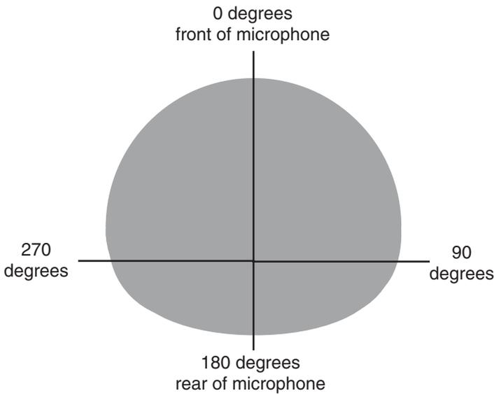
**Figure W.1** The wide cardioid polar pattern is more directional than an omnidirectional pattern, but it picks up more sound from the rear than a true cardioid pattern.
