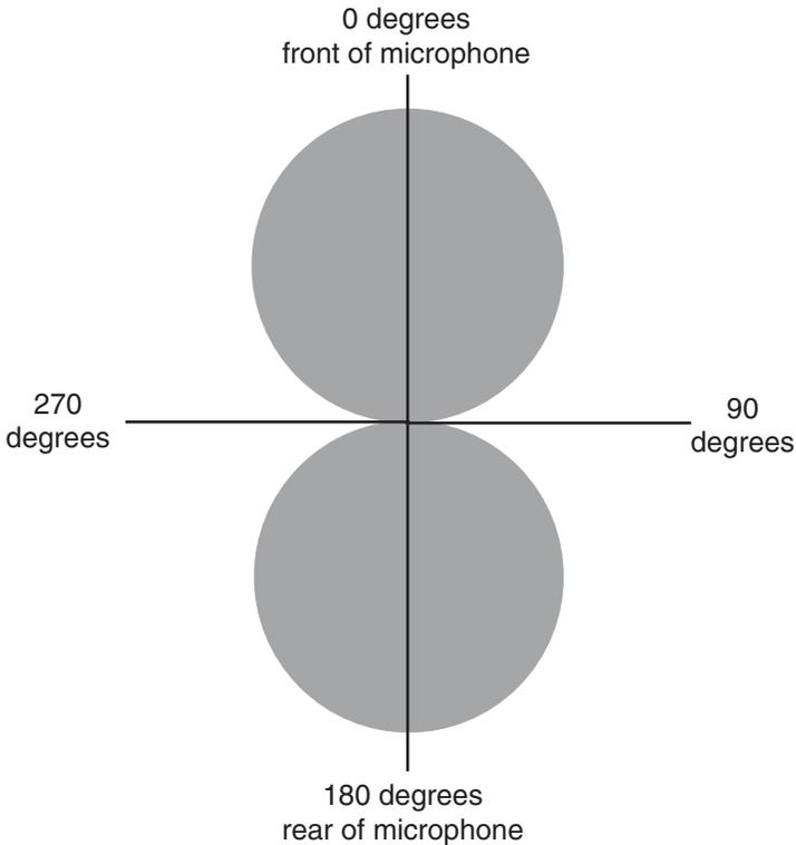
**Figure F.3** A figure-8 polar pattern consists of two spherical pickup lobes, one in front of the microphone and the other behind it.
