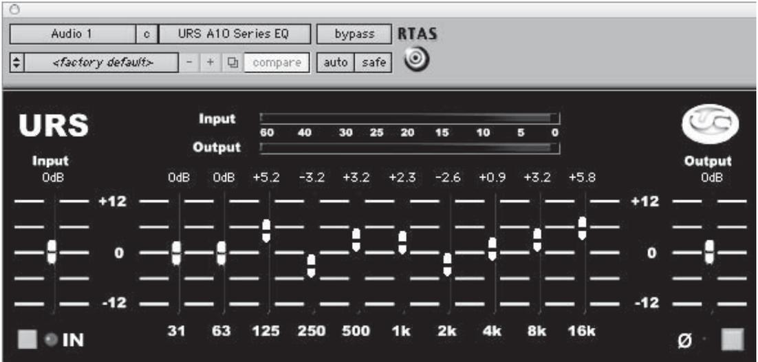
**Figure G.1** A type of equalizer that has a slider for the level of each band of frequencies, but that does not allow control over bandwidth or frequency center, is called a graphic equalizer.
