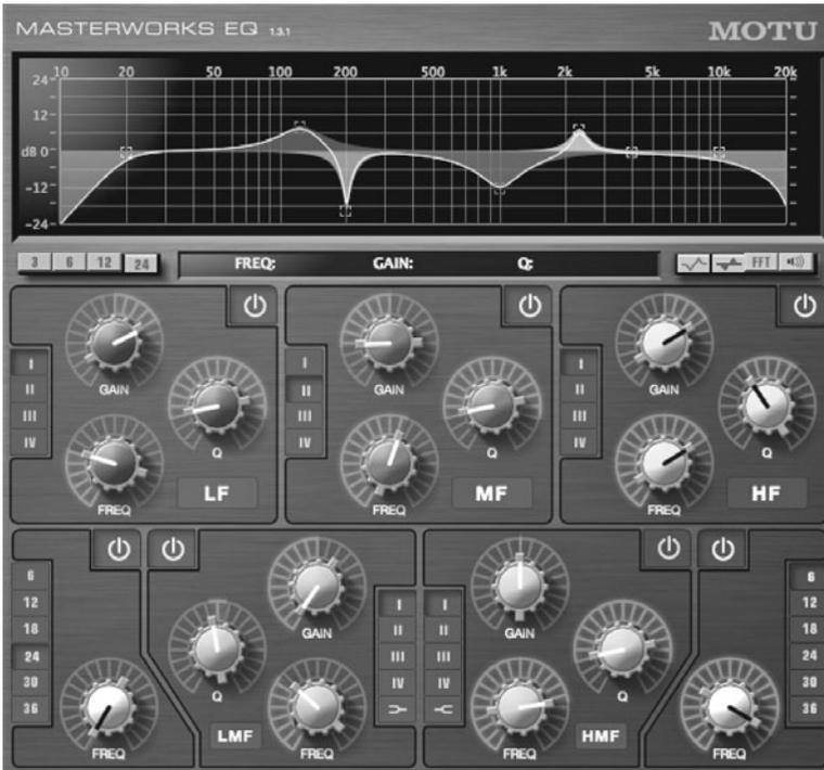
**Figure P.3** A parametric EQ allows control over the frequency, boost/cut, and bandwidth of each band.
