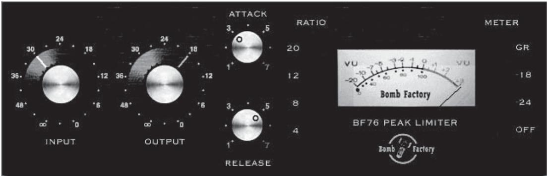
**Figure A.7** Pressing all four ratio preset buttons on an 1176-style compressor/limiter, such as this plug-in re-creation, results in a unique, punchy, overdriven sound.
