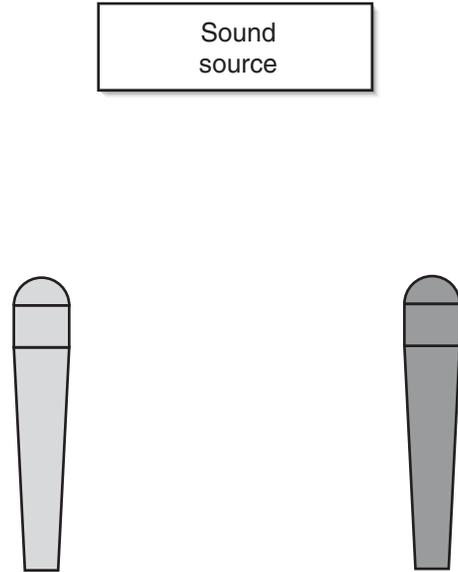
**Figure S.14** For the spaced-omni stereo miking technique, two omnidirectional microphones are positioned in parallel in front of the sound source, spaced several feet apart.
