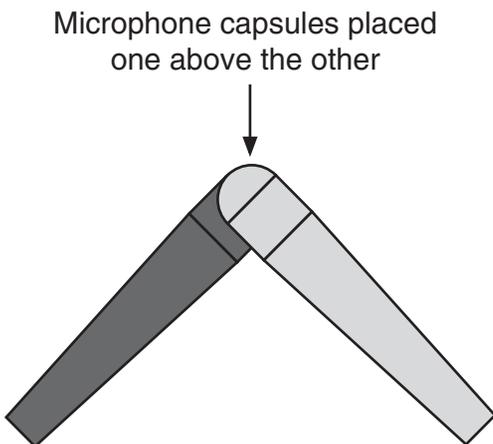
**Figure C.5** Coincident microphones are placed so their diaphragms are as close together as possible.
