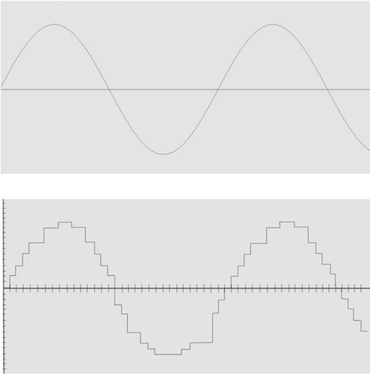
**Figure Q.1** Quantization represents a continuous signal with discrete steps.
