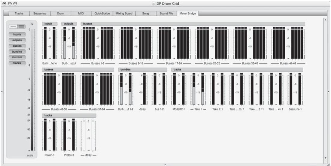
**Figure M.3** MOTU's Digital Performer DAW software offers a virtual meter bridge for displaying signal levels.
