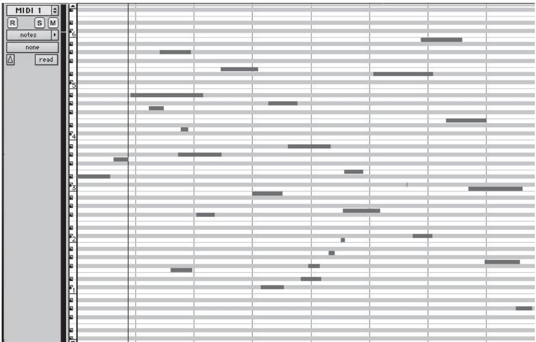
**Figure P.9** The piano roll editor in a sequencer is a graphic editor in which pitch, rhythmic placement, and note length can be edited, and notes can be inserted or deleted.
