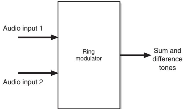
**Figure R.5** A ring modulator creates new sounds by generating frequencies that are at the sum and difference of the frequencies in two input signals.
