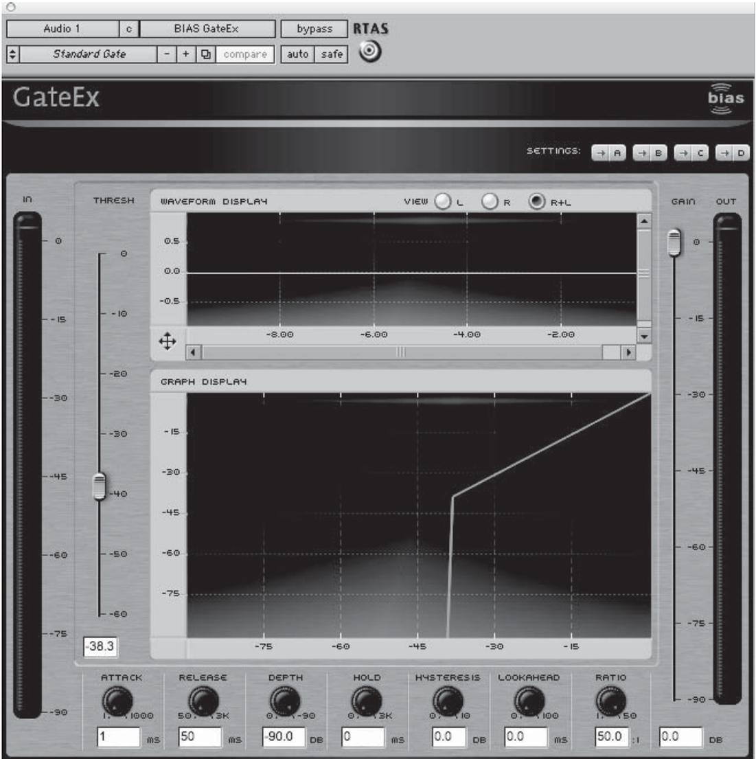
**Figure N.1** A noise gate opens when the desired signal crosses the threshold, allowing the signal to flow through. When the signal falls below the threshold, the gate closes, muting the output and silencing background noise.
