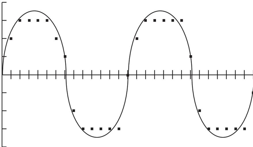
**Figure Q.2** Quantization error results from the difference between an actual value being measured and the discrete, quantized steps used to represent that measurement.
