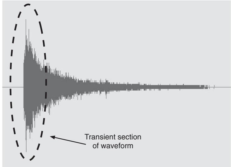
**Figure T.5** A transient is a quick spike in level, often found in the attack portion of a sound.
