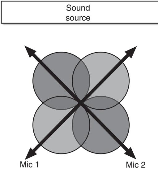
**Figure B.11** In a Blumlein pair, two figure-8 microphones are placed at 90 degrees to one another in front of a sound source. The result is a strong center image and good pickup of room ambience.
