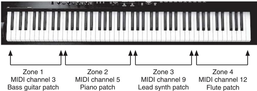
**Figure Z.4** Many keyboards can be split into zones, where each area of the keyboard can have its own assigned sound, MIDI channel, and other parameters. In many cases zones can overlap, allowing sounds to be layered.
