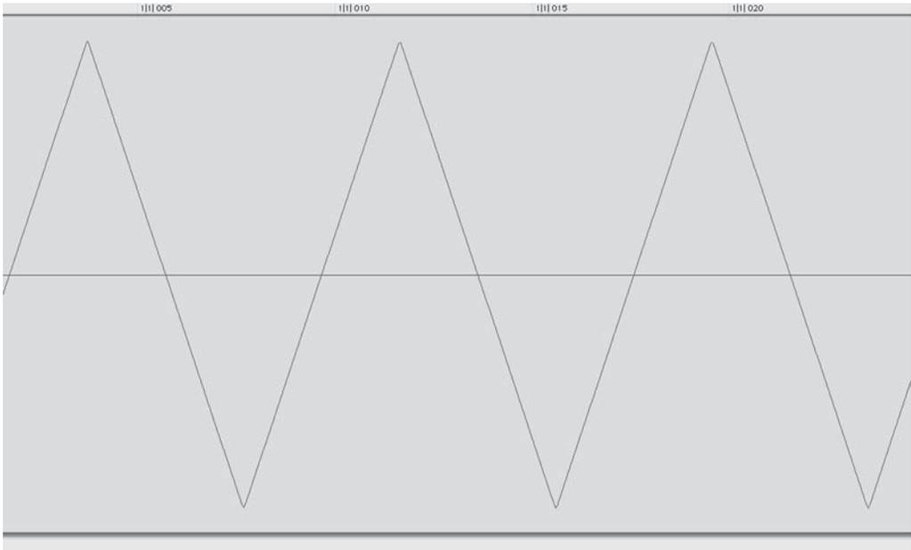
**Figure T.7** A triangle wave contains a fundamental frequency and odd harmonics.
