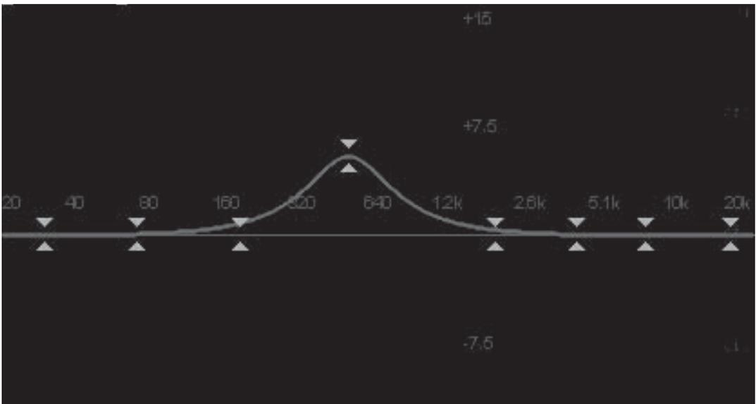
**Figure C.8** A constant Q equalizer maintains the same bandwidth for each band, no matter how much boost or cut is applied.
