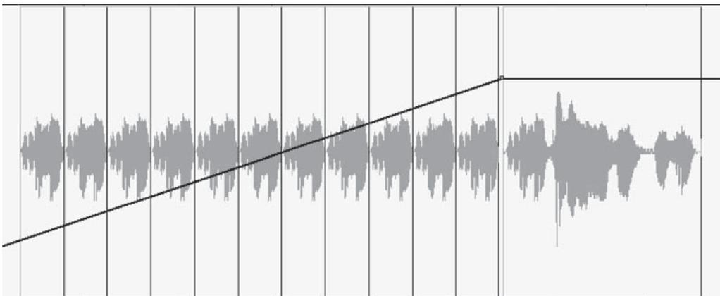
**Figure S.21** A stutter effect is created by repeatedly pasting a small slice of audio into a track. In this case, the first part of a word has been repeated, and a volume curve is used to fade it into the full word at the right.
