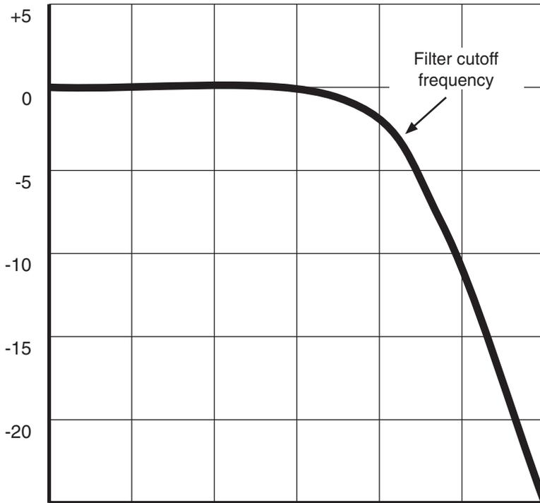
**Figure 5.10** The slope of a filter is the rate at which the frequencies past the cutoff are reduced in level.
