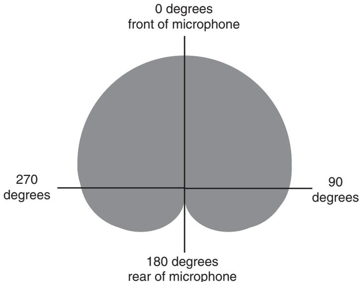
**Figure C.1** A cardioid polar pattern is heart-shaped, picking up sound best from the front and rejecting sound from the rear.
