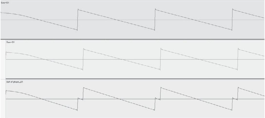
**Figure O.4** If two identical signals arrive at slightly different times, there will be phase cancellation problems. Note how different the bottom waveform, which was created by summing the top and middle waveforms, is from the original two waveforms—this is caused by the middle waveform being very slightly out of phase with the top waveform.
