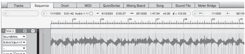
**Figure T.1** Tabs on a window in a computer program allow a user to select different views without opening an additional window.
