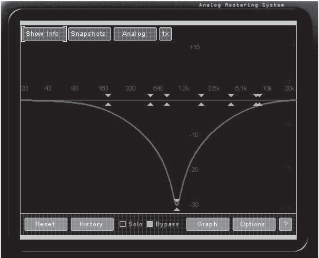
**Figure B.4** A band reject filter attenuates a central band of frequency, while allowing frequencies above and below the band to pass unaffected.
