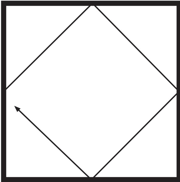
**Figure T.2** A tangential mode is caused by a sound wave reflecting across four surfaces in a room.
