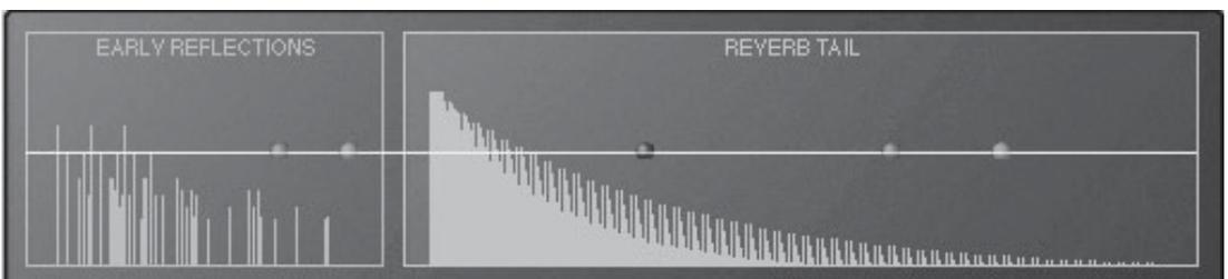
**Figure E.1** In a reverb processor, early reflections are very short delay-like repeats that simulate the acoustic reflections heard in a room.
