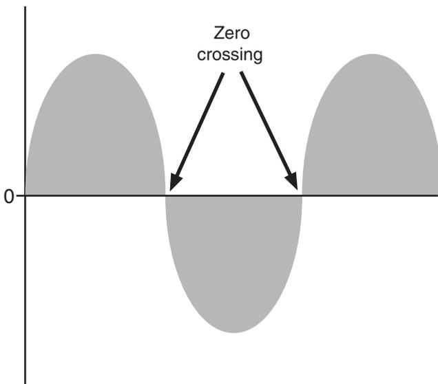
**Figure Z.1** A zero crossing is the point when the voltage in an analog waveform switches polarity.
