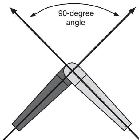
**Figure X.1** For XY stereo, two identical cardioid microphones are placed at 90 degrees to one another.
