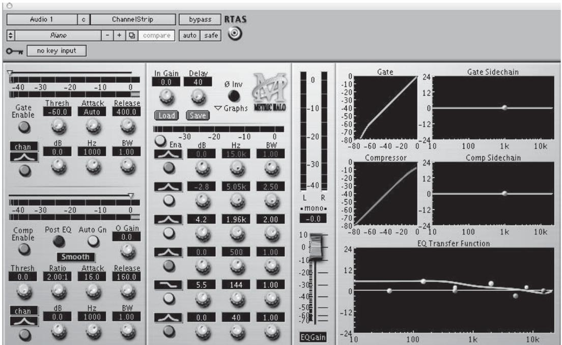
**Figure C.3** A plug-in channel strip contains a variety of processing in a single unit, such as EQ and dynamics processing—in this case, gating, compression, and equalization. A hardware channel strip would add a microphone preamp to the list of capabilities.
