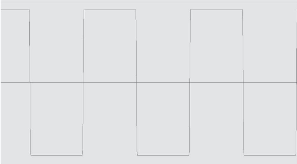
**Figure S.16** A square wave contains a fundamental frequency plus all odd integer harmonics. The ratio of high state to overall period is the duty cycle.
