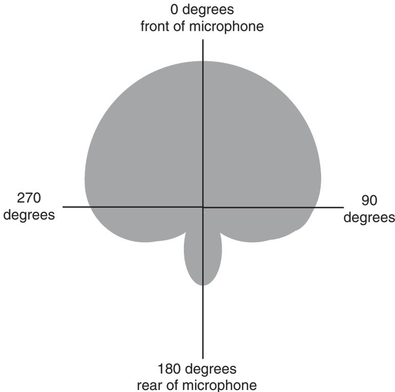
**Figure S.23** The supercardioid polar pattern is quite directional for good rejection of unwanted sound.
