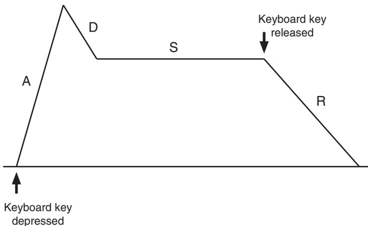
**Figure A.3** An ADSR has four stages—attack, decay, sustain, and release—that can be used to control synthesizer or sampler parameters, such as a sound's volume envelope.
