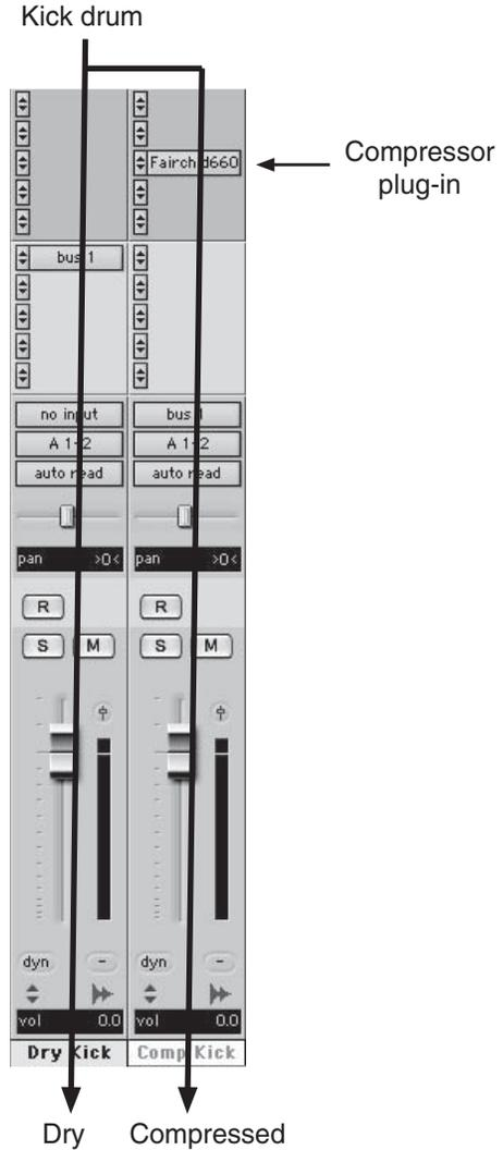
**Figure P.2** Parallel processing can be used to make a kick drum sound bigger. In this example, the kick signal is simultaneously being routed through a dry (unprocessed) mixer channel and through a compressor on another mixer channel. The dry and compressed channel outputs are combined, and the levels of the two signals are balanced to achieve the desired result.
