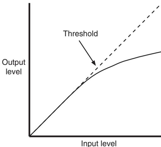
**Figure S.11** Soft-knee compression is less audible, especially with higher compression ratios.
