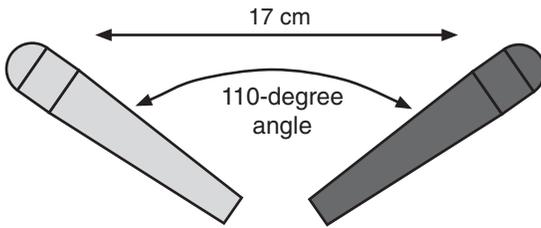
**Figure O.3** The ORTF stereo miking technique uses two cardioid microphones placed 17 cm apart at a 110-degree angle.
