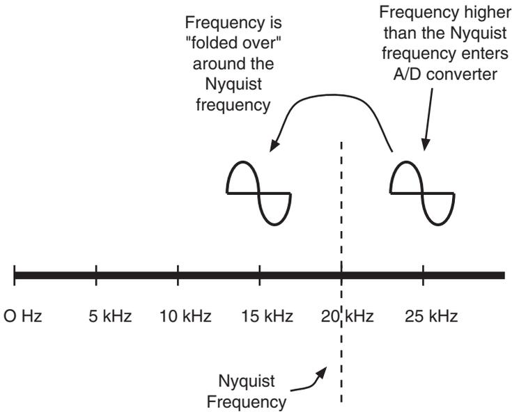
**Figure N.8** The Nyquist frequency is half the sample rate. If frequencies above the Nyquist frequency enter an analog-to-digital converter, they will be “folded over” around the Nyquist frequency, resulting in “alias” frequencies in the audible range. For this reason, analog signals are low-pass filtered before they are sampled in order to remove frequencies above the Nyquist frequency.
