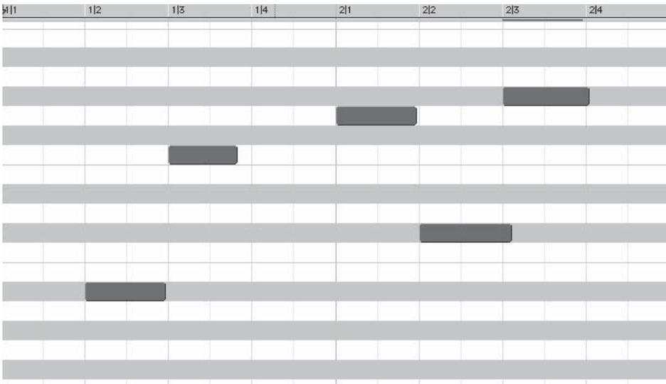
**Figure Q.3** Moving MIDI events to match a timing grid is called quantizing. The MIDI notes at the top have not been quantized; the bottom shows the same notes after they have been quantized to the grid.
