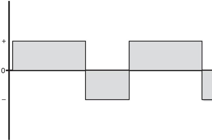
**Figure P.14** A pulse wave, or rectangular wave, has a duty cycle greater or lesser than 1:1.
