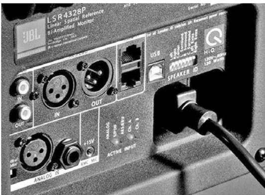
**Figure A.2** Active monitors feature built-in electronics including amplifiers, crossovers, and sometimes tone controls.
