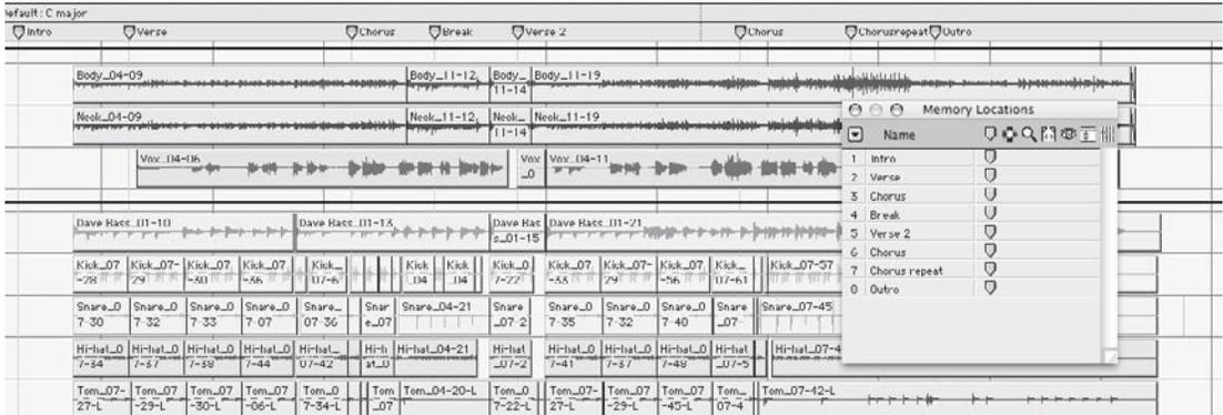
**Figure M.1** Markers (a.k.a. memory locations) can be used to store a location in a song in a DAW for quick navigation. The markers in this example are arrayed across the top of the tracks. The menu at the right can be used to locate the session to the selected marker.
