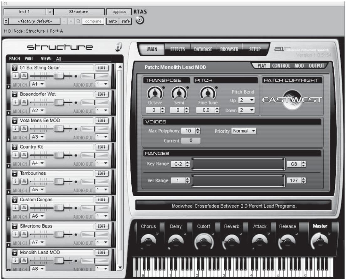
**Figure M.8** A multitimbral synth or sampler can be divided into virtual “parts,” each of which can have its own sound or preset and can respond to its own MIDI channel.
