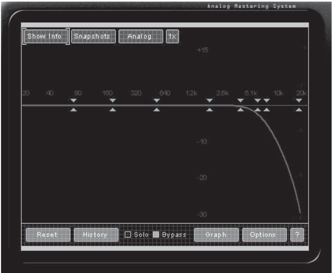
**Figure L.6** A low-pass filter reduces the level of frequencies above a certain point, while allowing those below to pass through unchanged.
