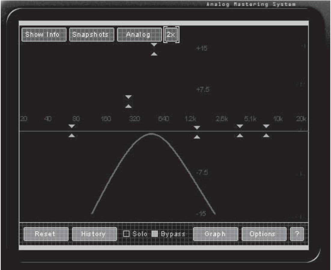
**Figure B.5** Bandpass filters allow only a certain range of frequencies to pass, while attenuating or rejecting all other frequencies.
