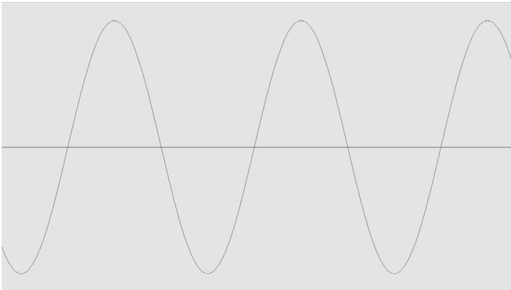
**Figure S.7** A sine wave is the simplest waveform, containing just a fundamental frequency without any harmonics.
