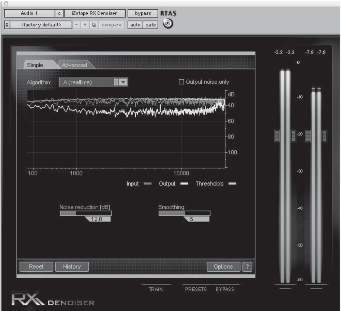
**Figure N.2** Some noise reduction software works by taking a “picture” of the noise, called a noise profile. The noise profile is used to determine what sonic material the software will consider noise in order to remove it from the overall signal.
