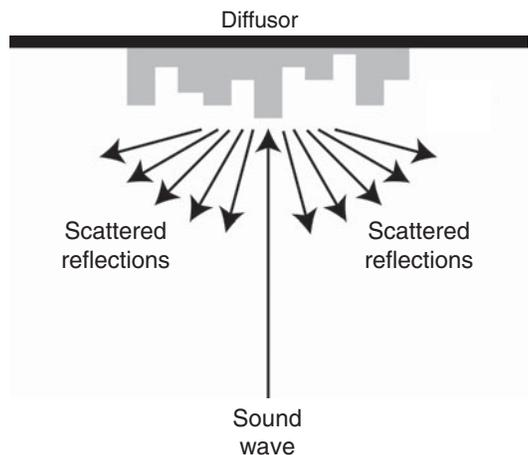
**Figure D.6** A diffusor breaks up and scatters reflections to reduce acoustic interference problems.
