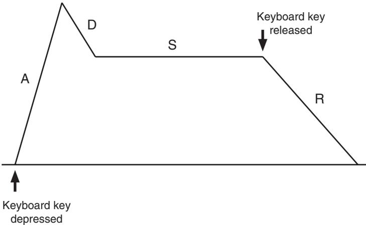
**Figure E.4** An envelope is a multistage control signal that can be routed to control the volume, pitch, or other parameter of a synthesizer or sampler sound.
