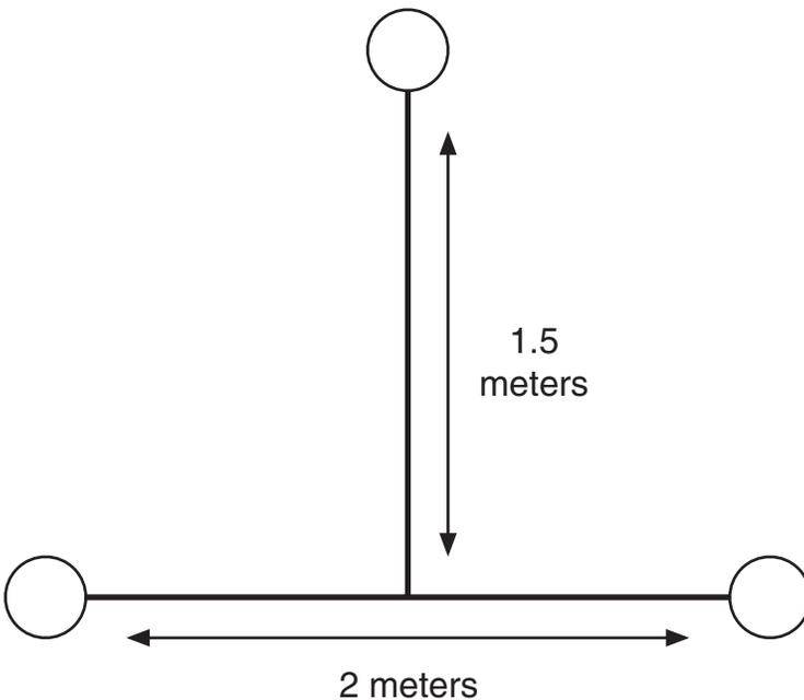
**Figure D.4** Decca Records developed the Decca Tree, a three-microphone stereo technique using omnidirectional microphones placed in a T arrangement.
