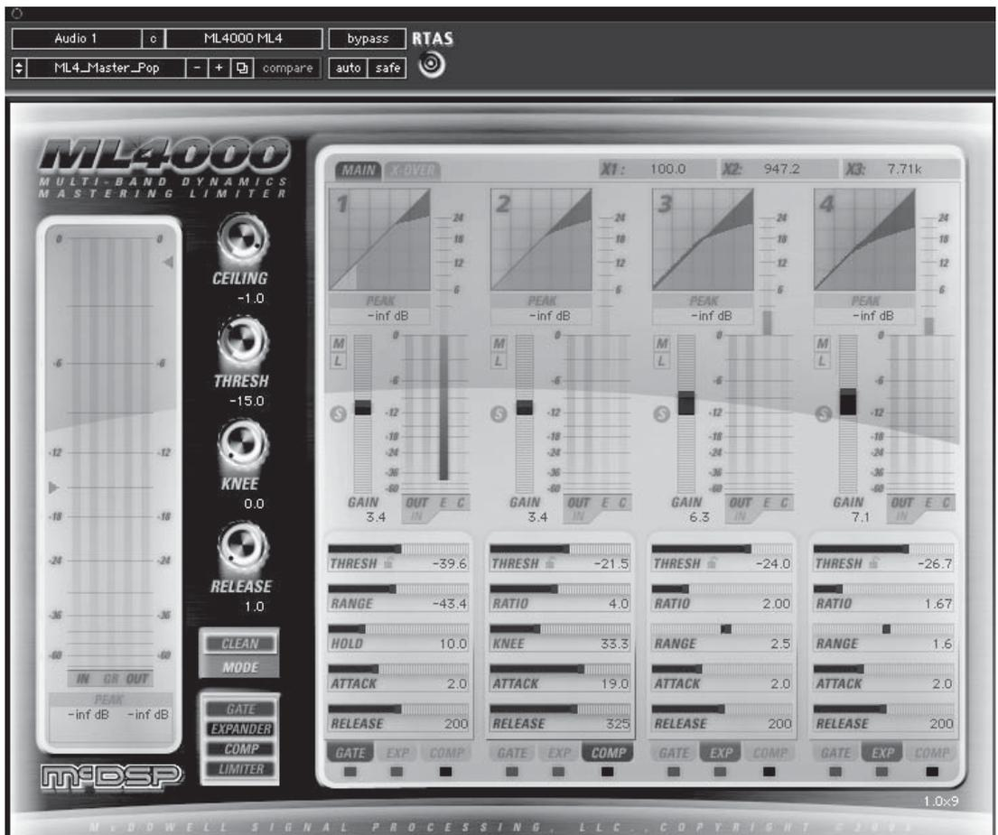
**Figure M.7** A multiband compressor splits the audio into separate bands of frequencies, each of which can be processed with an independent compressor.
