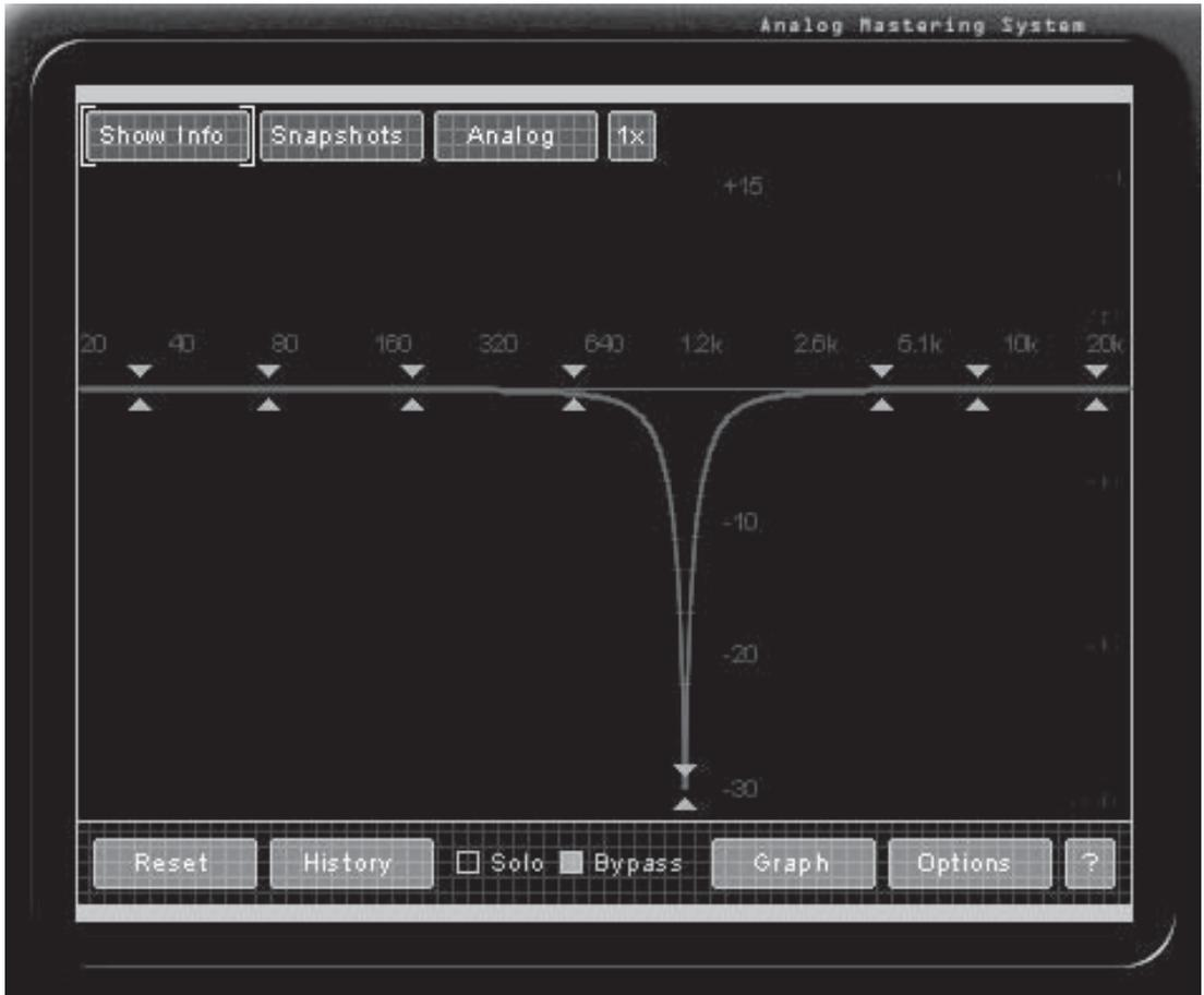
**Figure N.7** A notch is a narrow band of frequencies that has been reduced in level by a filter or other means.
