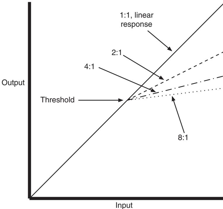
**Figure R.1** A dynamics processor's ratio control determines how much the output level will change compared to the input level.
