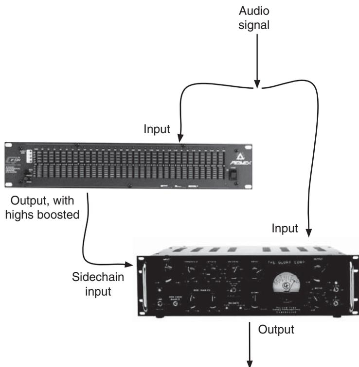
**Figure D.5** To create a de-esser from a compressor, route a signal to both the compressor’s audio input and its sidechain input. Use an equalizer to boost the high frequencies of the signal feeding the sidechain input.
