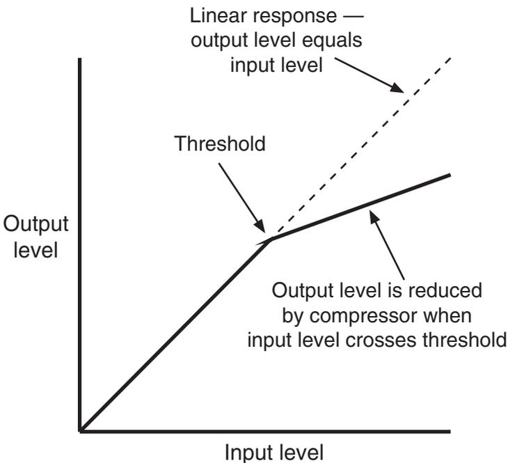
**Figure C.7** A compressor reduces the gain or level of a signal that exceeds a threshold.
