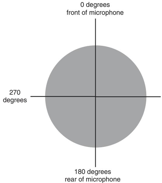
**Figure O.2** An omnidirectional microphone picks up sound equally well from all directions.
