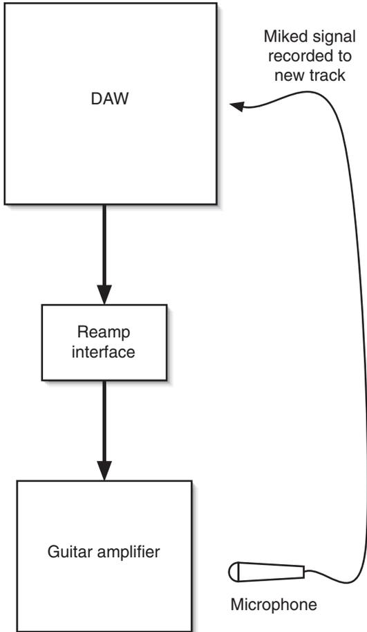
**Figure R.2** Reamping allows greater flexibility when deciding on guitar tones. A DI track is recorded, then is sent out through an amplifier and recorded to a new track.
