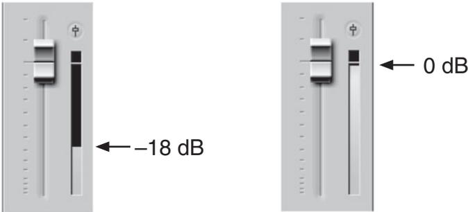
**Figure D.3** A digital meter reads 0 dB as the highest possible level before overload (right), unlike a VU meter. A signal that reads zero on a VU meter typically reads  $-18$  dB or  $-14$  dB on a digital meter (left). Many experts recommend  $-18$  as the best level for recording into 24-bit digital audio systems, as it allows plenty of room for clean transients.
