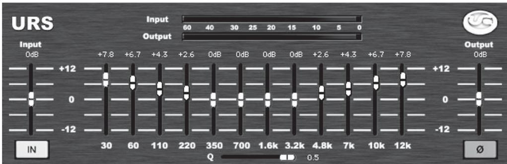
**Figure S.2** Cutting the midrange frequencies and either boosting or letting the high and low frequencies pass unchanged results in scooped mids.
