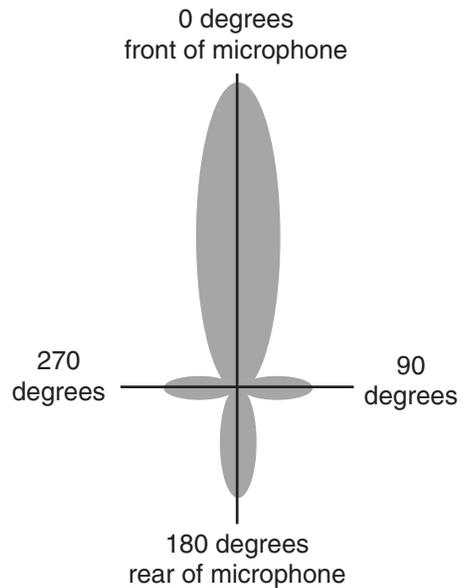
**Figure L.4** A shotgun microphone has a lobar polar pattern that can pick up distant sounds without interference from unwanted sounds.
