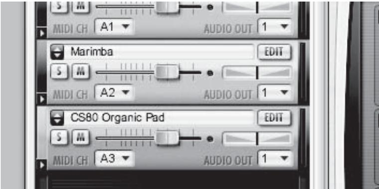
**Figure P.4** Each part in a multitimbral synthesizer can be set to produce a separate sound, on its own MIDI channel, with its own volume, pan, and other parameters.
