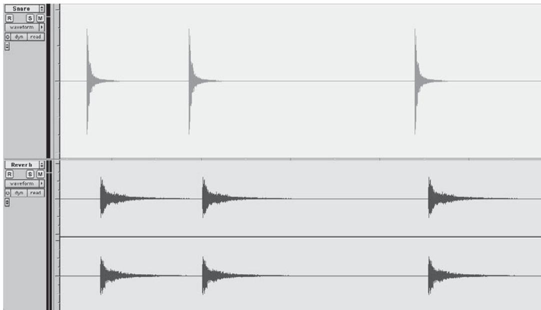
**Figure P.12** Pre-delay is the amount of time that elapses after a sound (a snare drum, in this case) and before the onset of reverb.
